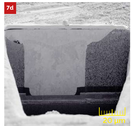
Fig. 7: (a and c) Curtaining can appear when milling at high ion beam currents. (b and d) Tilt-polishing with the Rocking Stage is an effective technique to get rid of the curtaining which results in smooth surfaces suited to perform failure analysis.
