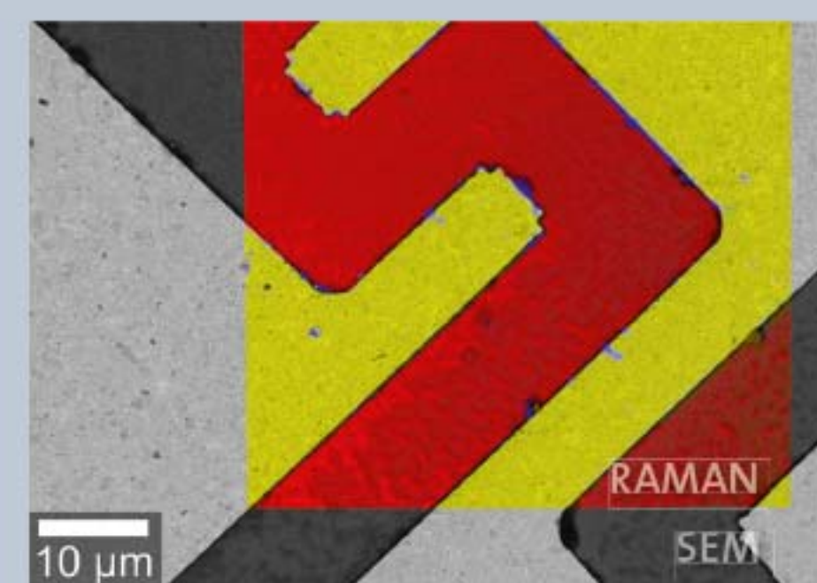
Raman-SEM image overlay of a LT GaAs sample. In the color-coded Raman image the gold substrate (yellow color) can be clearly distinguished from GaAs (in Red) correlated with the ultra-structure of the sample. Raman Image: 50 \mu\text{m} x 50 \mu\text{m} , 300 x 300 pixels = 90,000 spectra, 34 ms integration time per spectrum.
