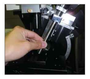
Residual stress in a micro area is measured by utilizing optional collimators. The collimators are easy to install and remove. Optional sizes are:  $\varphi$ 30 µm,  $\varphi$ 50 µm,  $\varphi$ 100 µm, as well as  $\varphi$ 300 µm,  $\varphi$ 500 µm,  $\varphi$ 2 mm, and  $\varphi$ 4 mm. Standard collimator sizes are  $\varphi$ 150 µm and  $\varphi$ 1 mm.
