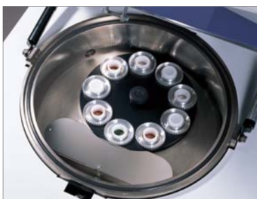
Optional sample spinner and 9-position changer allows analysis of non-uniform samples
