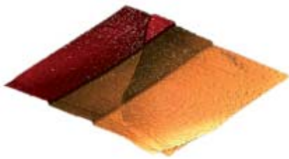
STM image of graphite surface. Image size: 800x800 nm
