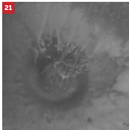
Fig. 21: Charging effects can severely damage the sample during FIB operations.
