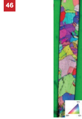
Fig. 45: 3D EBSD reconstruction of a Copper wire used in microelectronics. The volume 100 \times 100 \times 30 \mu\text{m}^3 was analysed within 2.5 hours using the XEIA3 Xe Plasma FIB-SEM. Crystal orientation was mapped using a colour coded inverse pole figure (IPF-Z). All scales in \mu\text{m} .
