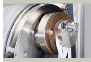
Fischione's history of innovation continues with the introduction of the next generation of ion source technology. Our patented TrueFocus ion sources are now optimized to perform at 100% ionization efficiency – the result is a highly efficient ion source that maintains a consistent beam current. This technology is built in to the Model 1051 TEM Mill.
