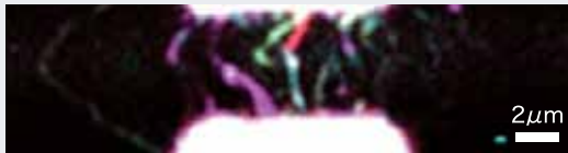
Raman image of RBM's distribution of SWNTs
