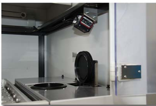
The barcode reader is positioned above the pre-evacuation chamber
