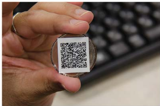
A two-dimensional barcode can be affixed to the non-analysis side of the sample
