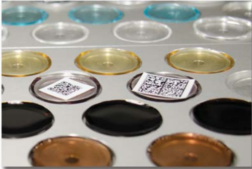
The sample deck can be configured to handle different sample sizes
